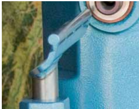
Newly designed tool rest with hardened round steel bar and Ø 30 mm stem. Extremely low-vibration.
