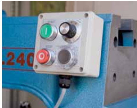
The inverter drive is mounted in a strong steel container, which can be wall mounted. All the lathe controls are grouped together in magnetic backed remote control box with 2m cable.
