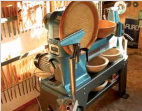
Fixing points for the approved VICMARC Outboard-Turning-Attachment. This allows the force put onto the toolrest to go directly to the floor.
