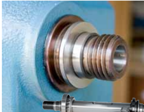
Hardened and precision ground spindle with No. 2MT and 15 mm through hole, with adjustable tapered roller bearings. M33 spindle thread inboard and outboard safety collar allows the safe use of disk sanders.
