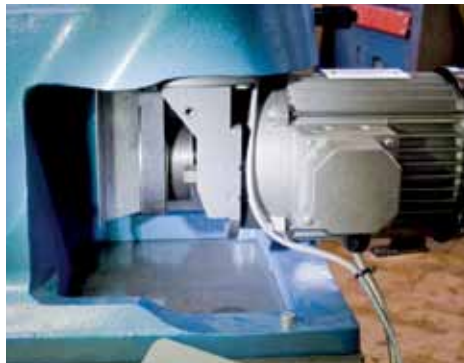
Another masterpiece from VICMARC! The motor is mounted low, below the level of the lathe bed in the most stable position, away from dust and shavings and also giving it a low centre of gravity.
