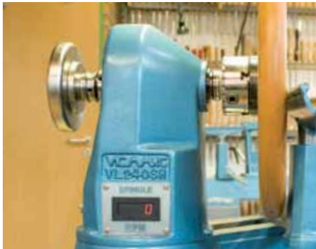
Ergonomical Headstock, Digital Readout shows true RPM
