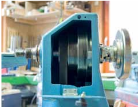
Three step pulleys for best torque 1. Step: 30 - 3000 rpm > normal operation 2. Step: 20 - 2000 rpm > big bowls 3. Step: 15 - 1000 rpm > heavy duty work
