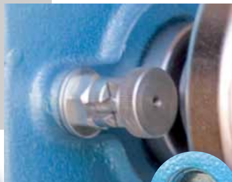
Spindle locking with integrated 24-hole indexing and sight glass
