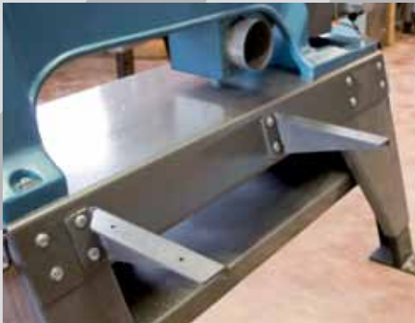
Dust extraction box with 100 mm connector could be hooked in the bed. 3 fixing points for mounting brackets for individually trays behind the lathe
