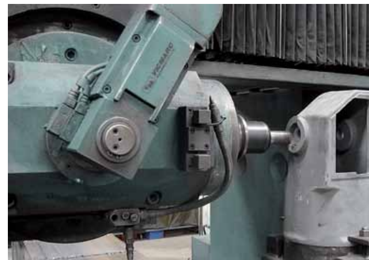
Milling of the seat for the conical roller bearing.
