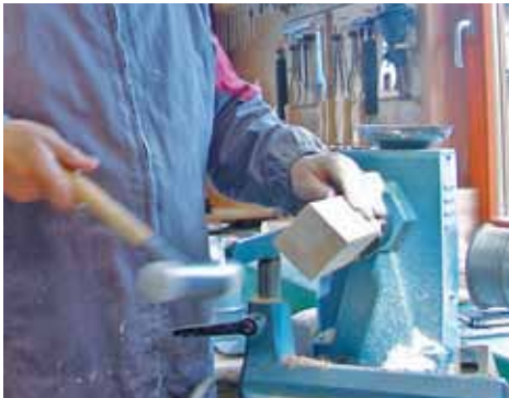
The taper roller bearings tolerate correcting strokes of hammer when using old German cup chucks.
