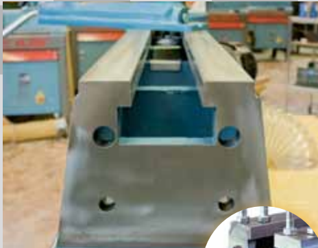
Precision machined face made from 22 mm cast iron for bolt on extension bed.
