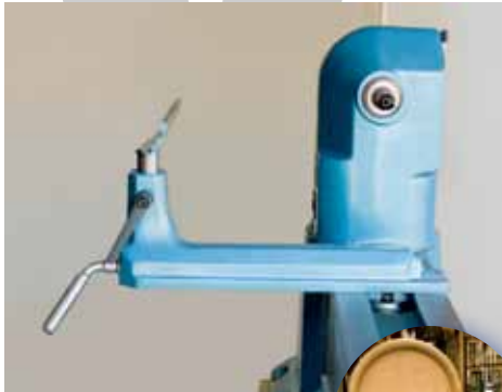
Extra long and solid cast iron banjo, for turning big bowls. (460 mm long, 150 mm height)
